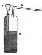
two mouths, as in the margin, put a number of small pieces of zinc, and a quantity of water sufficient to fill it about half full. Through a perforated cork fitted into one of the mouths of the glass, let a glass tube pass, grasped so tightly by the cork that no air can pass between them. This tube passes to near the bottom of the vessel. Its lower extremity terminates in a small opening, but its upper extremity is widened out into a fun-
